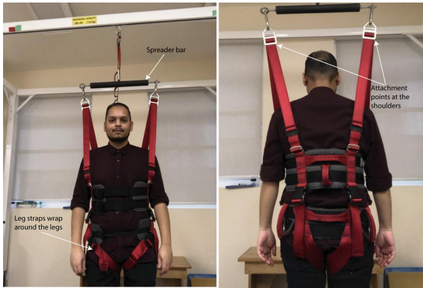
Figure 3.2. Example of a body-weight support harness.
